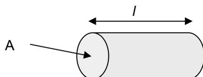
The diagram above shows a copper rod of length  $l = 0.080\text{m}$ , having a cross-sectional area  $A = 3.0 \times 10^{-4} \text{ m}^2$ .
